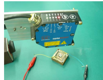
Fig. 11. Laser displacement sensor measures displacement signal.
