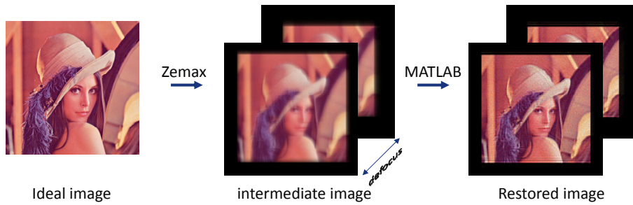
Figure 8. Imaging chain diagram associated with wavefront coded process by Zemax and decoded process by MATLAB program.
