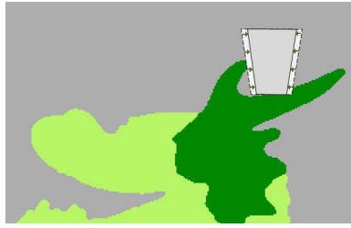
Fig. 13. When target layer (gray) is broken by the connection, the connection will be eroded horizontally to make the target layer continuous.
