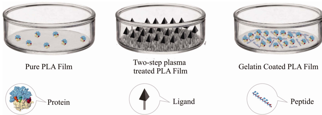
FIGURE 10. Sketches of the surface conditions of pure, two-step plasma treated and gelatin coated PLA films with immersed in culture medium. [Color figure can be viewed in the online issue, which is available at wileyonlinelibrary.com .]
