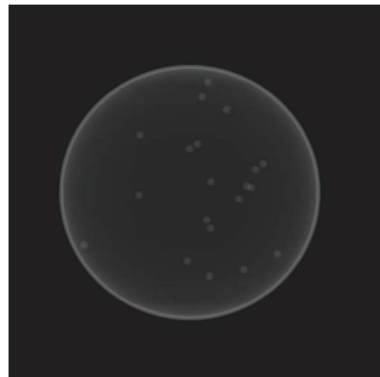
Figure 2. The simulated X-ray image of the phantom data. 180 emulated X-ray images were generated. The size of each image is 512×512 pixels, the rotation angle between two consecutive images is 1°, and the ranges of the vertical and horizontal errors are \pm 20 pixels. doi:10.1371/journal.pone.0084675.g002
