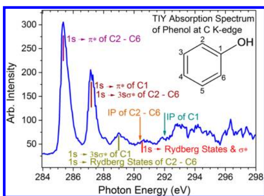
Figure 2. NEXAFS spectrum of phenol excited from 284 to 298 eV in a total ion yield mode. The scanning step was 50 meV, and the photon-energy resolution was 150 meV. The numbers of carbon atoms as well as the suggested assignments are exhibited. The ionization potentials of carbon atoms are also represented.
