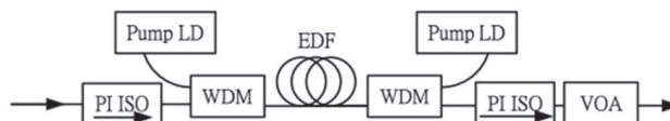
Fig. 1. Schematics of (a) supercontinuum generation system, (b) noise-like pulse laser, and (c) fiber amplifier. HNLF, highly nonlinear fiber; Pump LD, pump laser diode; WDM, wavelength division multiplexer; DCF, dispersion compensation fiber; PC, polarization controller; PD ISO, polarization-dependent isolator; EDF, erbium-doped fiber; PI ISO, polarization-independent isolator; VOA, variable optical attenuator.
