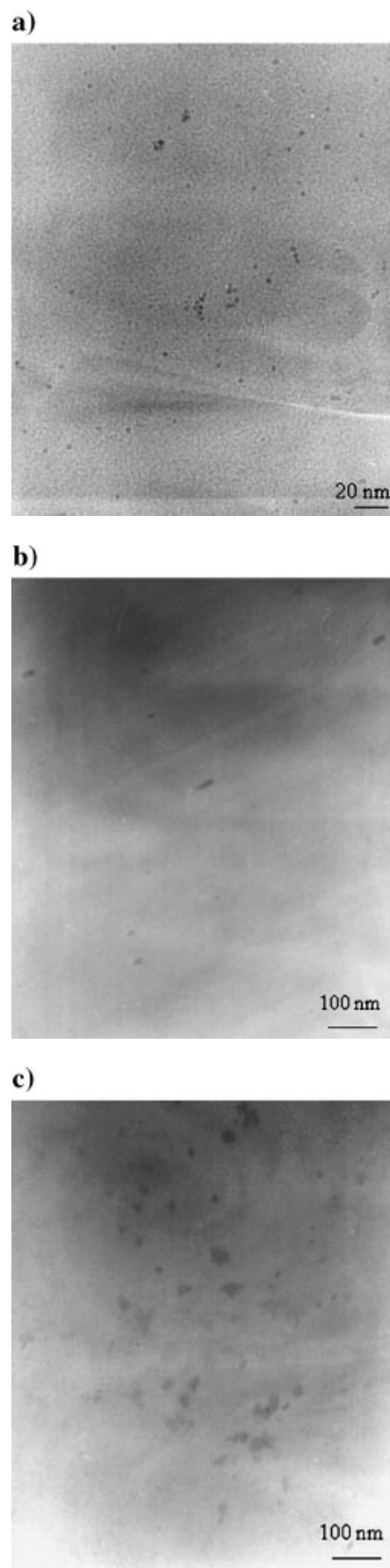
Figure 11. TEM images of (a) TPM-stabilized ZnO nanoparticles, (b) BTDA-ODA/ZnO-5 wt.-%, and (c) PMDA-ODA/ZnO-5 wt.-% hybrid films.
