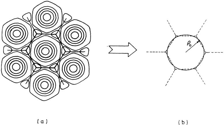
FIG. 2. The hexagonal unit cell of the triangular flux-line lattice [shown in (a)] is replaced by a circular unit cell with an equal area [shown in (b)].
