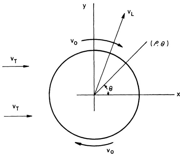
FIG. 1. A single vortex moving with a velocity  $V_L$  is driven by a uniform transport flow  $V_T$ . The circulation of a stationary vortex outside of a normal core is  $V_0$ . The polar coordinate  $(\rho, \theta)$  is used.
