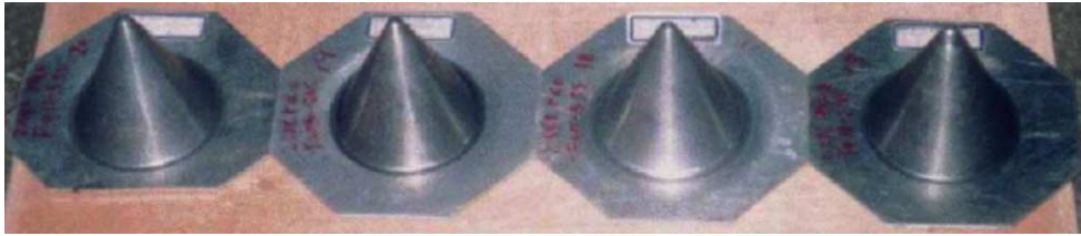
Fig. 4. Spun cones from four independent shear spinning experiments.
