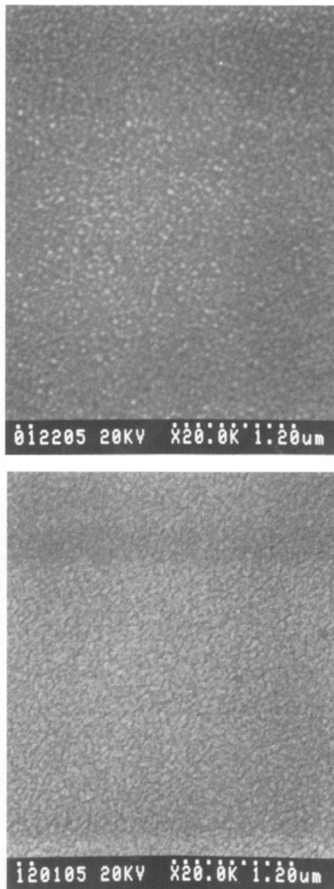
Fig. 7. SEM micrographs of (a, top) Co (surface) and (b, bottom) TEOS oxide surface for the \alpha -Si/Co (40 Å)/TEOS oxide/Si sample annealed at 800°C.
