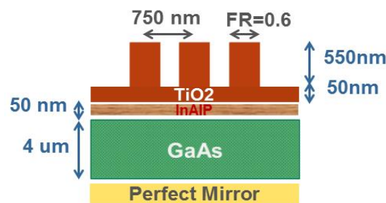
Fig. 1. The cross-section view of 4um GaAs solar cells we simulate here.
