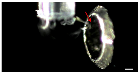
Figure 1. Photograph obtained when ejecting a liquid droplet from a pipette tip close to the orifice of a mass spectrometer applied with -4000 V. Scale bar, 150 \mu\text{m} . The red cursor indicates the formation of Taylor cone. This figure is available in colour online at wileyonlinelibrary.com/journal/jms .
