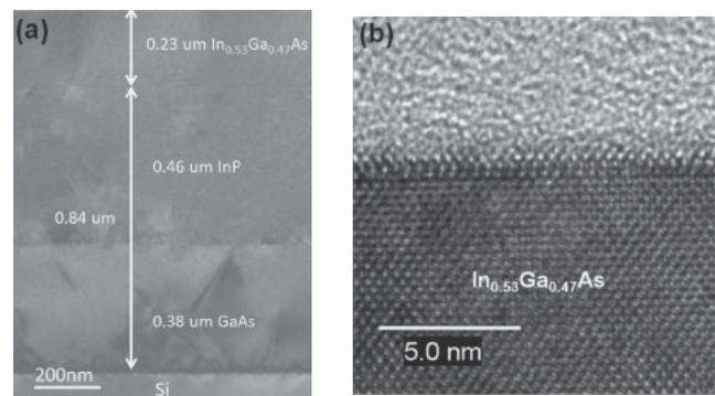
**Fig. 1.** (a) Cross-sectional TEM image of  $\text{In}_{0.53}\text{Ga}_{0.47}\text{As}$  heterostructure on Si. The metamorphic GaAs/InP buffer in this work has a total thickness of 0.84  $\mu\text{m}$ . (b) High-resolution TEM image of top InGaAs channel.
