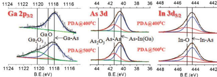
**Fig. 3.** XPS spectra of Ga  $2p_{3/2}$ , As 3d, and In  $3d_{5/2}$  after  $\text{Al}_2\text{O}_3/\text{In}_{0.53}\text{Ga}_{0.47}\text{As}$  was annealed at  $400$  and  $500^\circ\text{C}$ ; the Si doping concentration of the n- $\text{In}_{0.53}\text{Ga}_{0.47}\text{As}$  layer is  $1.7 \times 10^{17} \text{ cm}^{-3}$ .
