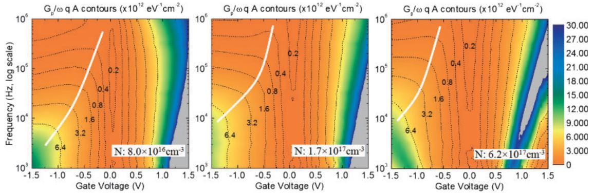
**Fig. 6.** Normalized parallel conductance contour map for  $8.0 \times 10^{16}$ ,  $1.7 \times 10^{17}$ , and  $6.2 \times 10^{17} \text{ cm}^{-3}$  Si-doped  $\text{n-In}_{0.53}\text{Ga}_{0.47}\text{As}$  MOS capacitors with PDA temperature of  $400^\circ\text{C}$ . The lines indicate the local  $G_p/\omega$  maxima and trace of surface Fermi level.
