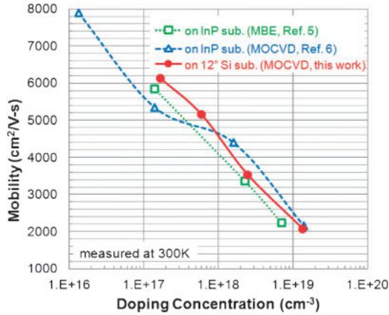
**Fig. 2.** Hall mobility of  $\text{In}_{0.53}\text{Ga}_{0.47}\text{As}$  as a function of doping concentration. The  $\text{In}_{0.53}\text{Ga}_{0.47}\text{As}$  layers were grown on InP by MBE and MOCVD.
