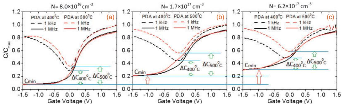
**Fig. 4.**  $C/C_{\text{max}}-V$  curves at 1 kHz and 1 MHz for (a)  $8.0 \times 10^{16}$ , (b)  $1.7 \times 10^{17}$ , and (c)  $6.2 \times 10^{17} \text{ cm}^{-3}$  Si-doped n- $\text{In}_{0.53}\text{Ga}_{0.47}\text{As}$  MOS capacitors with PDA temperatures of  $400$  and  $500^\circ\text{C}$ .
