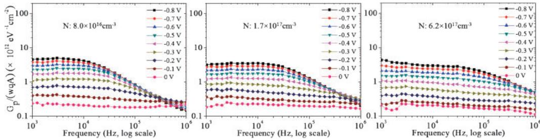
**Fig. 7.**  $G_p/wqA$  ( $A$ :  $1.96 \times 10^{-5} \text{ cm}^2$ ) vs frequency curves at different gate biases after  $400^\circ\text{C}$  PDA for  $8.0 \times 10^{16}$ ,  $1.7 \times 10^{17}$ , and  $6.2 \times 10^{17} \text{ cm}^{-3}$  Si-doped  $\text{n-In}_{0.53}\text{Ga}_{0.47}\text{As}$  MOS capacitors.
