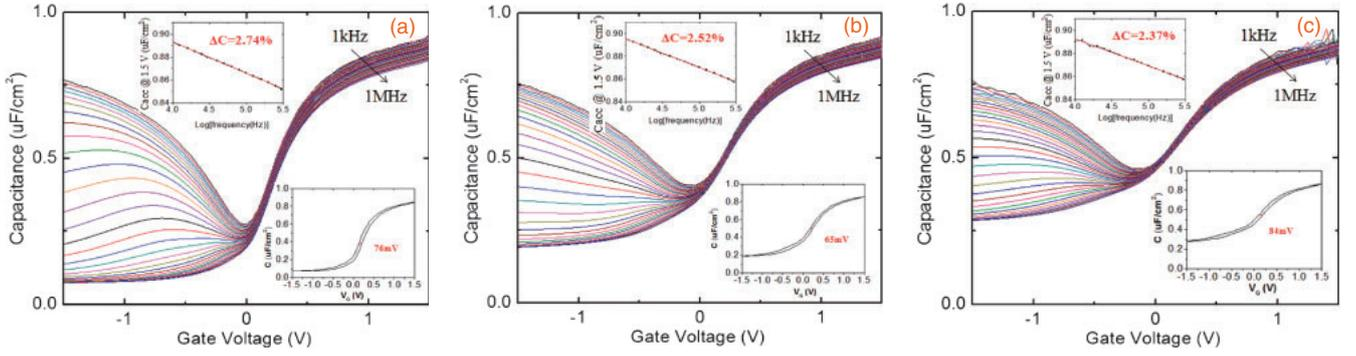
**Fig. 5.**  $C$ - $V$  curves for (a)  $8.0 \times 10^{16}$ , (b)  $1.7 \times 10^{17}$ , and (c)  $6.2 \times 10^{17} \text{ cm}^{-3}$  Si-doped  $\text{n-In}_{0.53}\text{Ga}_{0.47}\text{As}$  MOS capacitors with PDA temperature of  $400^\circ\text{C}$  (diode area  $A$ :  $1.96 \times 10^{-5} \text{ cm}^2$ ).
