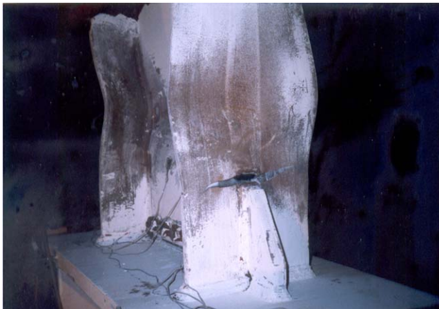
Fig. 19. Specimen SR30 after failure.
