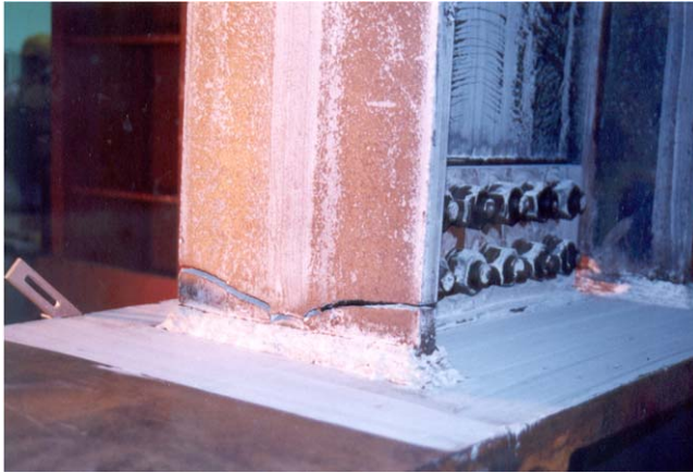
Fig. 6. Yielding and fracture of the beam flange of specimen S6.
