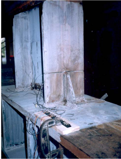
Fig. 20. Specimen SR20 after failure.
