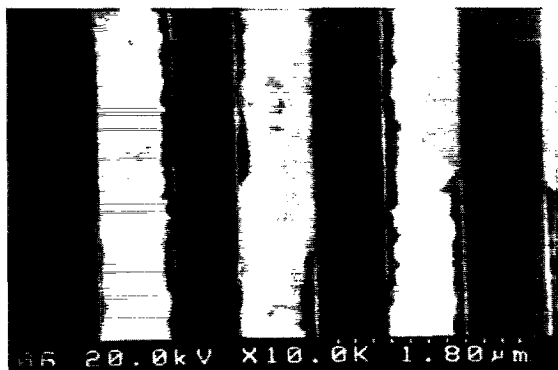
Fig. 8. Scanning electron micrographs showing a serious corrosion of tungsten resulting from a 120 s post-CMP cleaning in a 5% ammonia solution.
