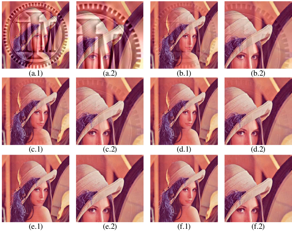
Fig. 7 The visual quality comparison for different \delta value of watermarked Lena images. (a.1), (b.1), (c.1), (d.1), (e.1) and (f.1) are watermarked Lena images for \delta=0, 0.5, 0.7, 1.0, 1.2, 1.5 respectively. (a.2), (b.2), (c.2), (d.2), (e.2), and (f.2) are close-up images of (a.1), (b.1), (c.1), (d.1), (e.1), and (f.1) respectively. The PSNRs of (a.1), (b.1), (c.1), (d.1), (e.1), and (f.1) are 17.43 dB, 28.86 dB, 32.52 dB, 36.21 dB, 37.67 dB and 39.11 dB respectively
