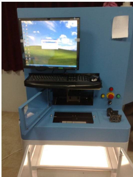
Fig. 2 The outlook of the realized optical lens test bench machine
