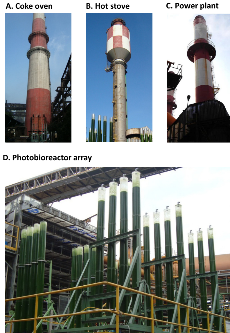
Fig. 1. The sources of the flue gas from the furnace of a coke oven (A), hot stove (B) or power plant (C) at the China Steel Corporation, Taiwan. The outdoor photobioreactor array for microalgal culturing is adjacent to the furnace (D). The photobioreactors are cylindrical and composed of acrylic polymer. The columns are 300 cm in length and 16 cm in diameter. The working volume of each photobioreactor is 50 L and the total volume of the photobioreactor array is 1200 L, i.e., the content of 24 photobioreactors.
