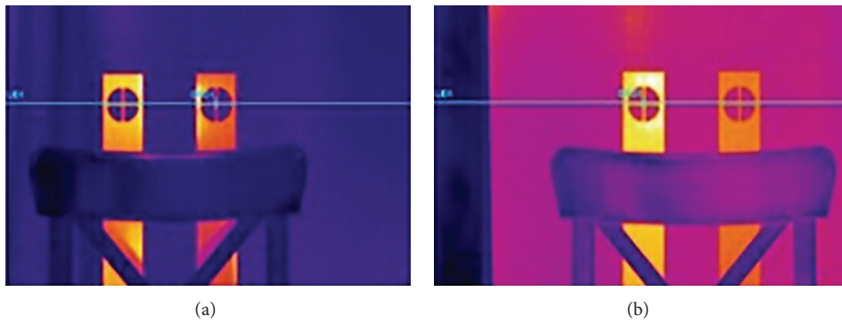
FIGURE 2: The different capture image effect (a) alignment image for MIR camera; (b) alignment image for LIR camera.
