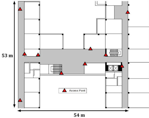
Fig. 5. Map of the experimentation site (53 m \times 54 m). The gray region comprising the main hall and hallways is the area of interested and feasible area for robot traveling. The red triangles indicate the areas equipped with off-the-shelf APs; their locations are assumed to be unknown.
