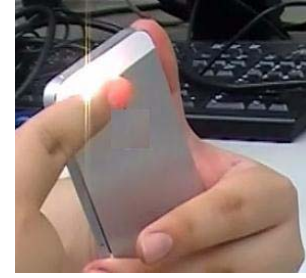
Fig. 4. Fingertip PPGs measured by a CMOS camera in a smart phone.
