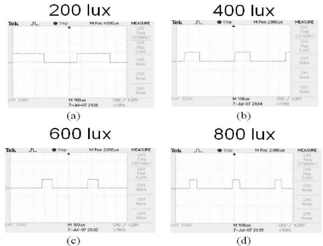
Fig. 6. Measurement results of the oscilloscope traces of the designed light-to-frequency converter under the illuminance at (a) 200 (b) 400 (c) 600 (d) 800 lux.
