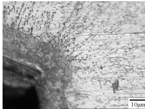
(a) SEM micrograph of the cross-section of a nickel micro mould insert. (The dark part at the lower left corner is a cavity left by removing the base plate.)
