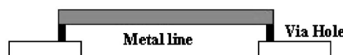
Figure 1. Testing structures consisted of metal chains 3.5 \mu\text{m} wide and 55 \mu\text{m} long and via hole 0.5 \mu\text{m} wide interconnected by differing arrays for stress migration.
