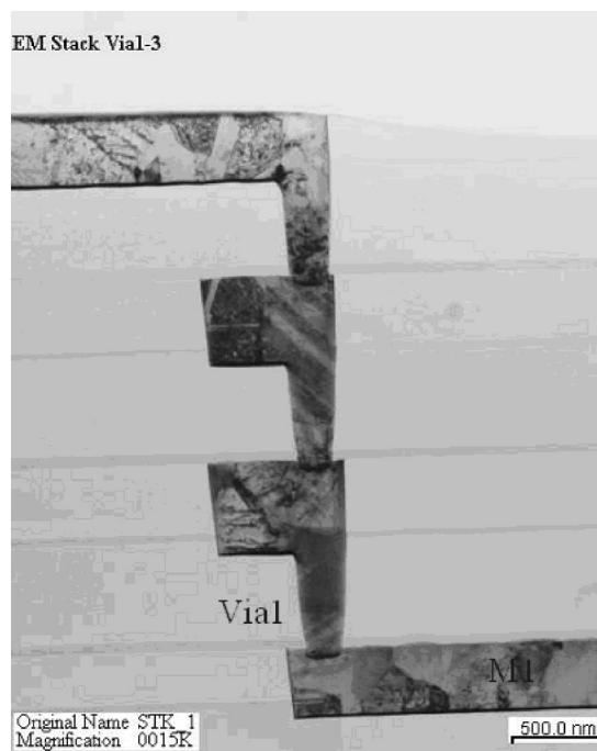
Figure 15. Stack via under TEM shows that it is void free.
