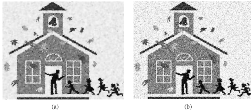
Fig. 12. (a) Original image and (b) grayscale image captured by the test chip under the light intensity of 0.57 \text{ mW/cm}^2 and V_{\text{com}} of 1.79 \text{ V} .
