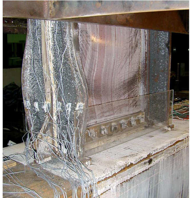
Fig. 16. Local buckling of beam flange and web of specimen BR105SB.
