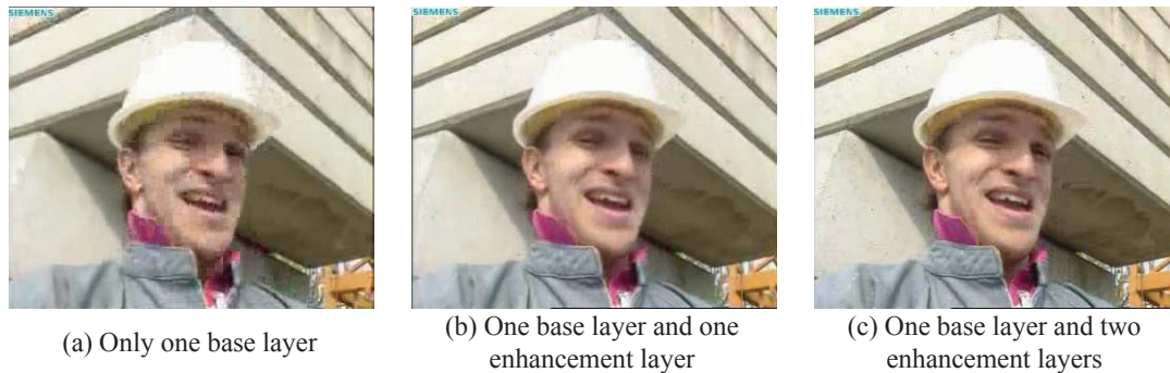
Figure 2 The video quality for the MSS under various numbers of video layers (the video, foreman, is downloaded from the video trace library [27]). (a) Only one base layer. (b) One base layer and one enhancement layer. (c) One base layer and two enhancement layers.
