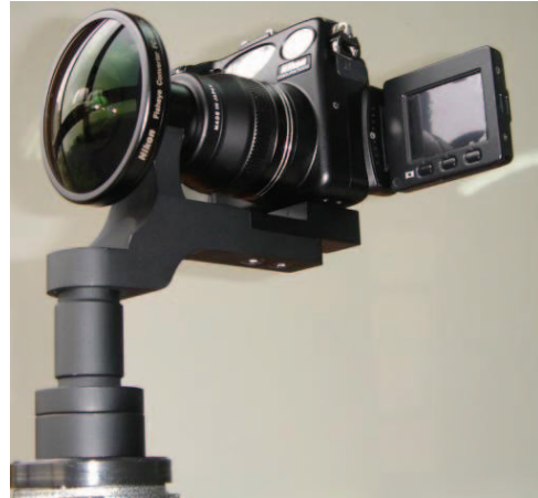
Fig. 10. The self developed pano head and 183 degree fisheye lens for creating the spherical panorama images
