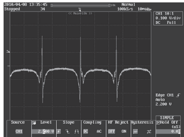
Fig. 14. Measurement of focusing error signal (S-curve).
