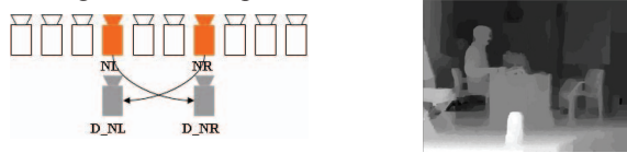
Fig. 2. Left: stereo camera setting, right: depth map estimated from stereo camera setting.
