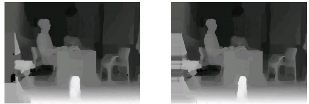
Fig. 7. Result of the depth refinement. Left: depth map before refinement, right: depth map after refinement.
