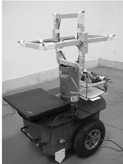
Figure 2. Digital microphone array mounted on the robot.
