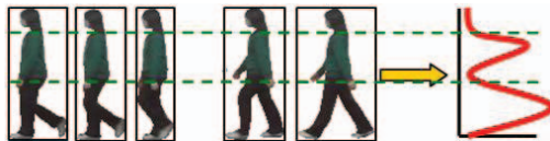
Fig. 3. The constituent components of a posture are partitioned based on local variance extraction.
