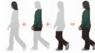
Fig. 4. A new posture is composed of three components (head, body, and legs).
