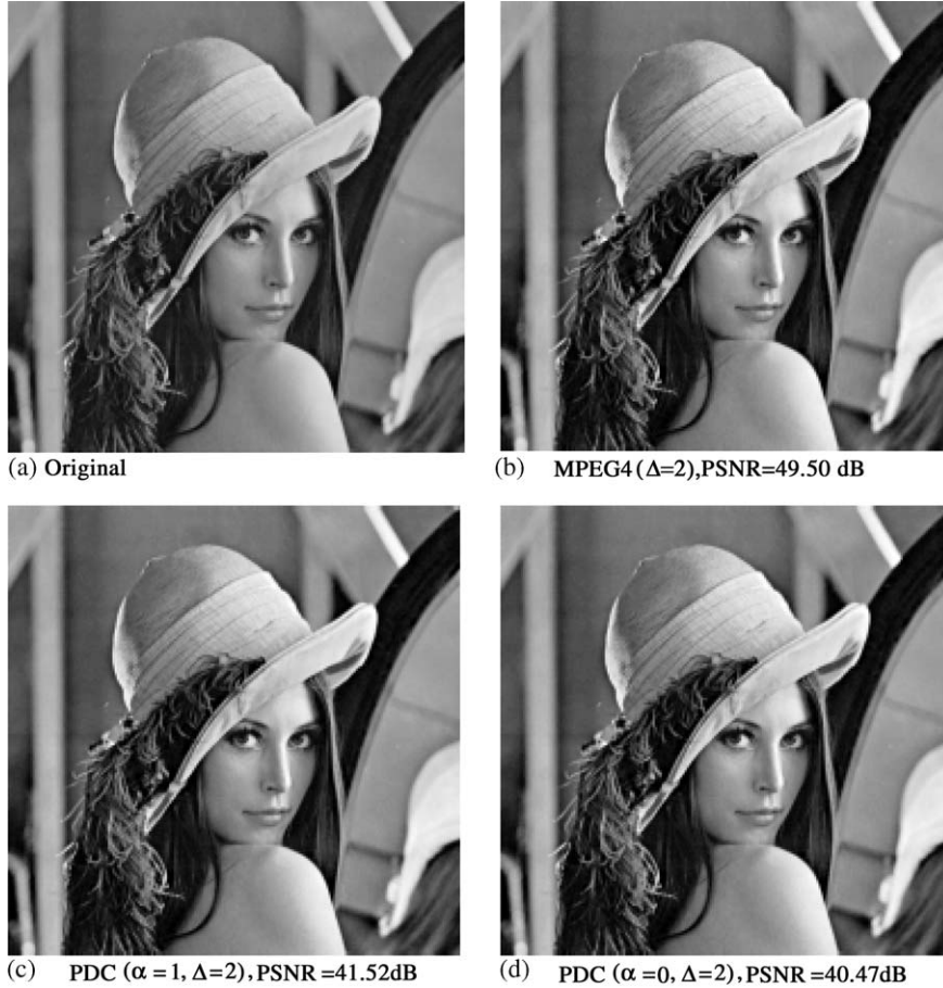
Fig. 5. The reconstructed image of size 512 \times 512 and in grayscale format, namely Lena, using MPEG-4 VTC and the proposed perceptual dithering coding. The quantization step size ( \Delta ) used is 2 and the two weighting values ( \alpha ) are used for the perceptually dithering. It should be noted that these images have been verified to be visually indistinguishable from the original image under the same viewing environments where the psychovisual model is created as described in Section 2.
