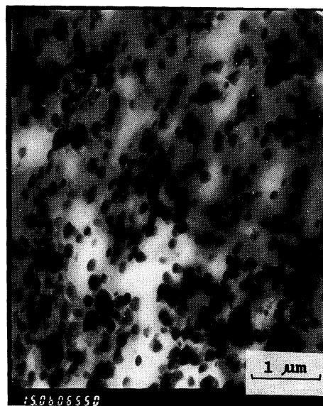
Figure 7. TEM micrograph of PC15/ABS2/MBS = 50/7.5 blend.
