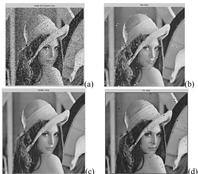
Fig.11. Simulation results of 2-D application: (a) image with impulsive noise (b) image with 3rd-order filtering and N=3 (c) image with 5th-order filtering and N=3 (d) image with 7th-order filtering.
