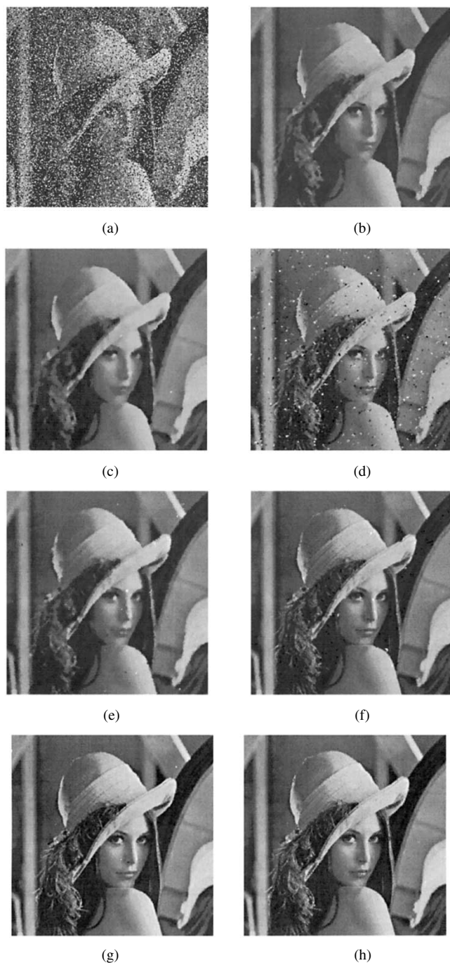
Fig. 2. (a) Image “Lena,” corrupted by impulse noise of p = 0.3 . Filtered images using (b) 3 \times 3 median, R = 1 ; (c) 5 \times 5 median, R = 0 ; (d) 3 \times 3 CWM; k = 1 , R = 1 ; (e) 5 \times 5 CWM; k = 2 , R = 0 ; (f) 3 \times 3 SD-ROM, R = 1 ; (g) 3 \times 3 ours, R = 1 ; (h) 5 \times 5 ours, R = 1 .
