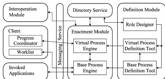
Fig. 6. Architecture of the prototype system.
