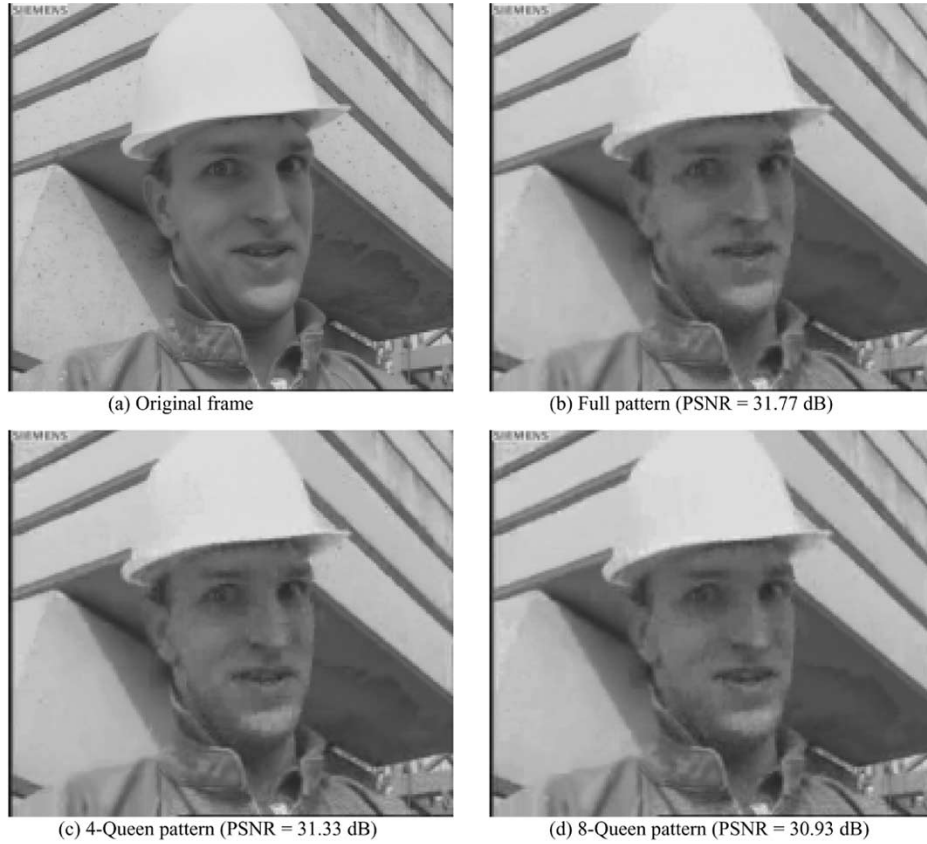
Fig. 8. Reconstructed Y components for the 102nd frame of the Foreman sequence in CIF format. (a) The original frame. (b)–(d) Constructed pictures with Full Search and N-Queen patterns.
