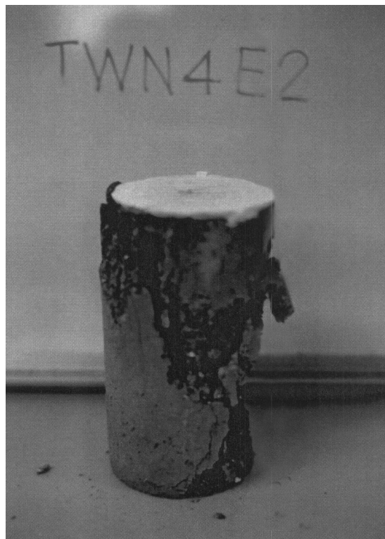
Fig. 15. Failure mode of typical specimen (with steel fiber) at 800°C
