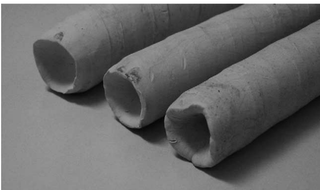
Fig. 13. End cavity of the rolled workpiece.
