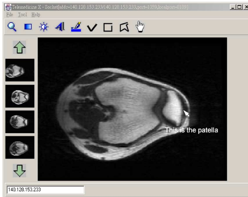
Fig. 1 A displayed MR knee image during consultation. The synchronous cursor or pointer is pointing out the patella. An annotation is indicated in the image. The connected site is exhibited by the IP address shown in the left bottom of the window.
