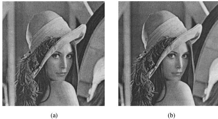
Fig. 3. Experimental results of embedding randomly generated decimal digits ( 512 \times 512 digits and each digit is 0–9) in Lena: (a) is the resulting image obtained by the simple LSB method, (b) is the resulting image obtained by the proposed method. Notably, m = 10 here, and thus m is not a whole power of 2.
