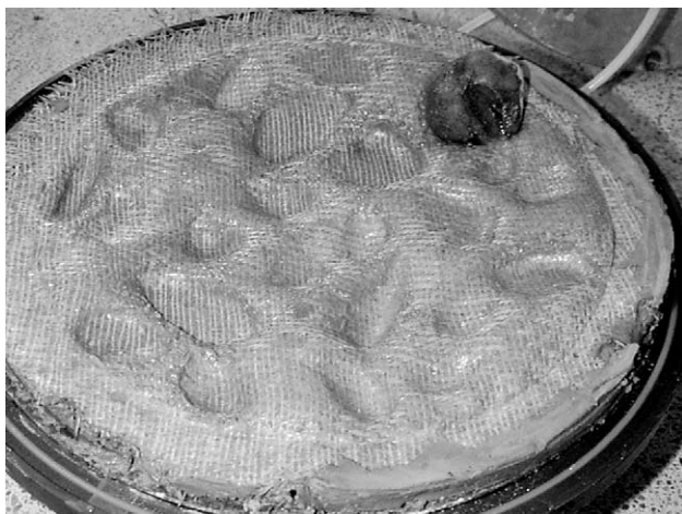
Fig. 10. Specimen GCL-B-4 after permeability test.
