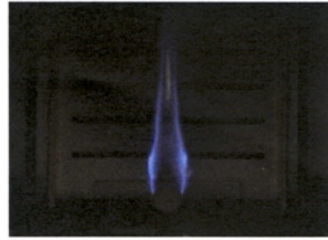
(C2) Wake flame ( U_{in}=1.2\text{m/sec} )
