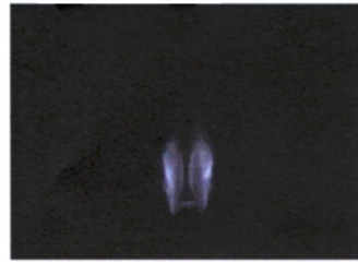
(C4) Late wake flame ( U_{in}=1.43\text{ m/s} )
