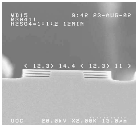
Fig. 3. The cross-section of the stable suspended InP/airgap DBRs captured by SEM.
