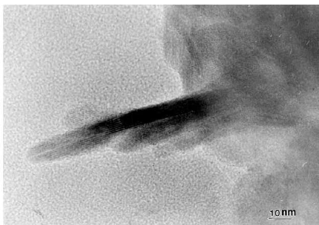
Fig. 7. High-resolution TEM image in the needlelike particle of cd-HA crystal.
