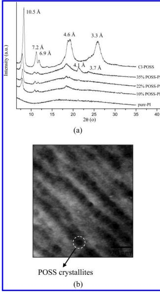
**Figure 3.** (a) X-ray diffraction curves of POSS/polyimide nanocomposite films. (b) Transmission electron micrograph of a cross section of POSS–polyimide nanocomposite film.
