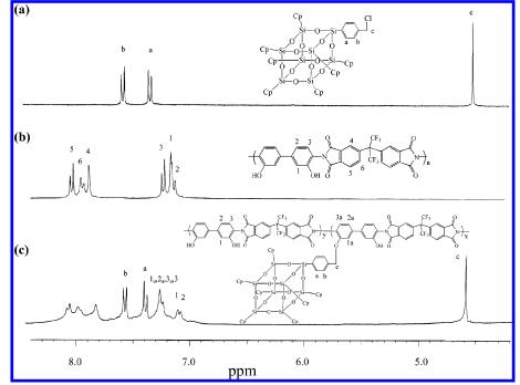
Figure 1. <sup>1</sup>H NMR spectra of (a) Cl-POSS, (b) hydroxyl polyimide, and (c) 35% POSS-polyimide.
