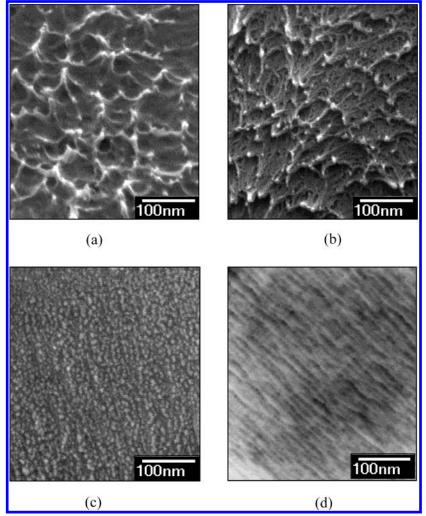
**Figure 4.** Field-emission scanning electron micrographs of the fractured surface of (a) 10 mol %, (b) 22 mol %, and (c) 35 mol % POSS–polyimide nanocomposites. (d) Transmission electron micrograph of a cross section of a 35 mol % POSS–polyimide nanocomposite film.
