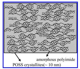
**Figure 5.** Schematic drawing of the architecture of polyimide-tethered POSS.
