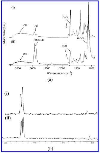
**Figure 2.** (a) FTIR spectra of (i) hydroxyl polyimide and (ii) 35% POSS–polyimide. (b) <sup>29</sup>Si NMR spectra of (i) Cl–POSS and (ii) 35% POSS–polyimide.
