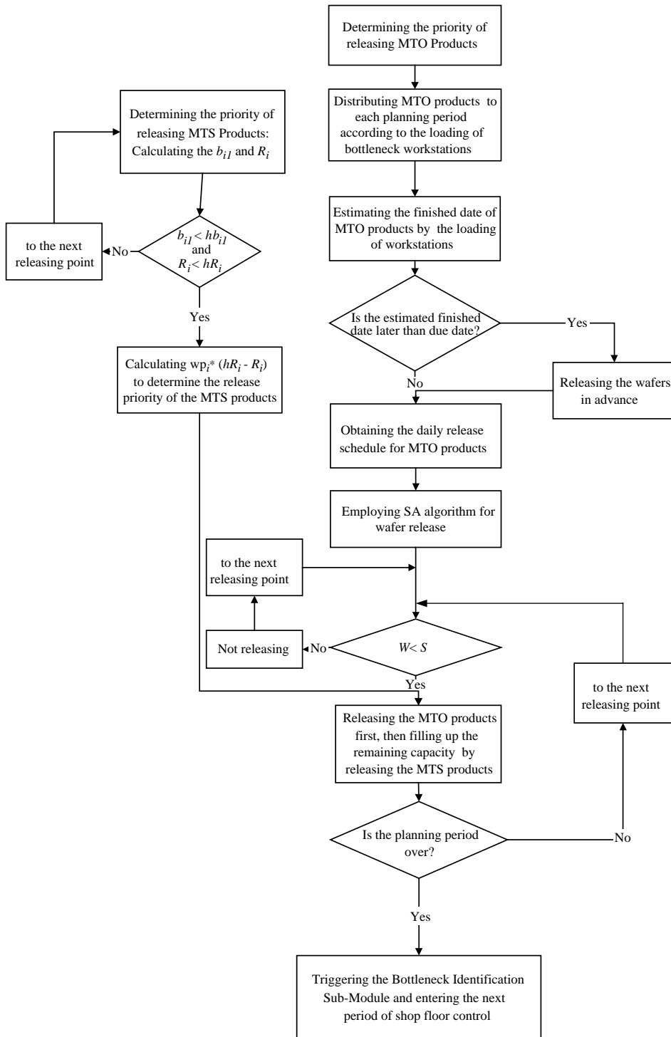
Fig. 2. The flow of order releasing sub-module.
