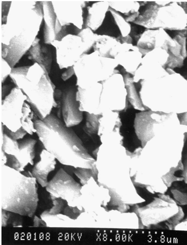
Fig. 3. The \text{SiC}_p powders with irregular polygonal shape.
